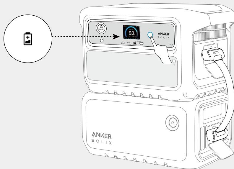
If you need to disconnect the power station from the expansion battery during use, press the on/off button of expansion battery for 3 seconds to turn it off. Then unplug the charging cable.
