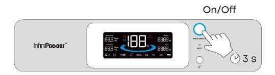
Press the main power button for 3 seconds to turn your power station on or off. When the "Battery Level" icon shows on the LCD screen, your power station is ready to charge devices.
