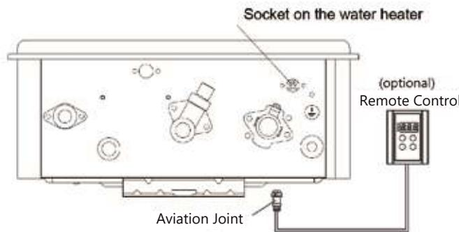
2. For two controls: First, cut off the aviation joints on the two controllers, plug one into the socket on the water heater (length is dependent on your requirements), and throw away the other. Then connect the wires of the aviation joint to the inlet wire of the connector, and connect the two remote control to the outlet wires of connector.
