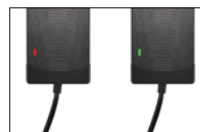
Red: charging Green: full of charge
